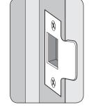
NB The plunger beside the latchbolt deadlocks the latchbolt and protects it against manipulation. IT MUST NOT enter the strike plate aperture when the door is closed.
