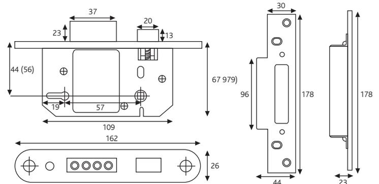
All dimensions are in mm and are nominal. Numbers in brackets relate to 3" version of lock. Diagram illustrates product in locked position. ERA reserves the right to change specification without notice. It is the responsibility of the door manufacturer to ensure that the finished product meets any required safety and performance specification.
